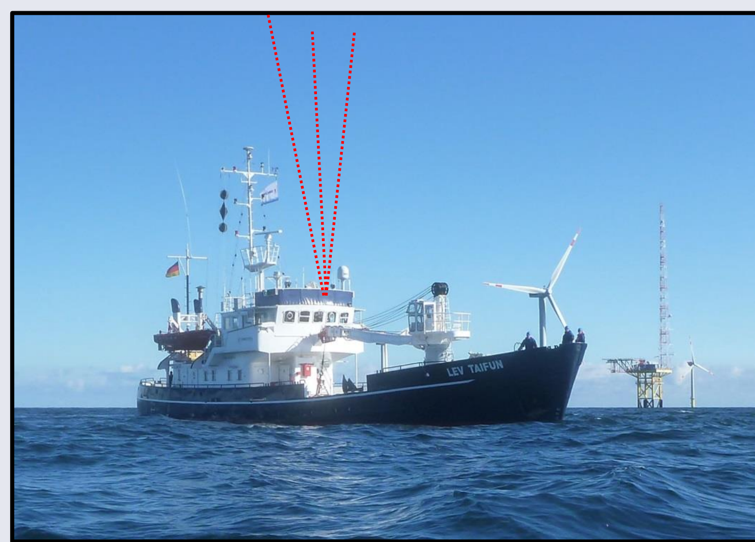
Figure 2: Ship-lidar measurement in proximity to offshore meteorological mast FINO1. Position of the lidar system is indicated by the red beam lines.
